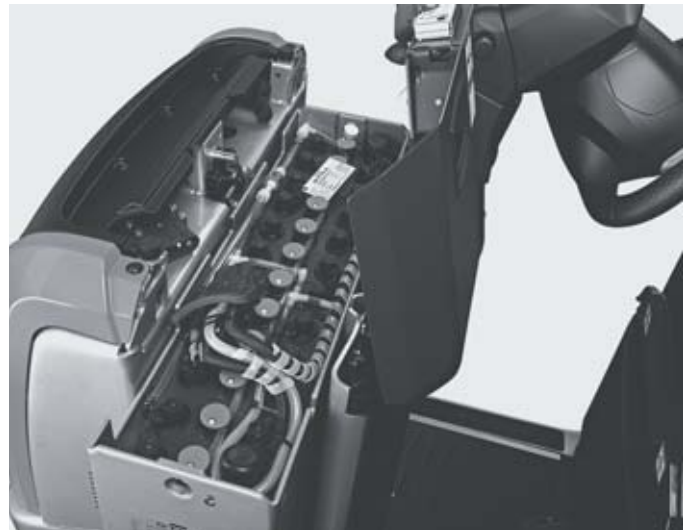
Optional side battery changes guarantee maximised availability and best user/driver ergonomics
