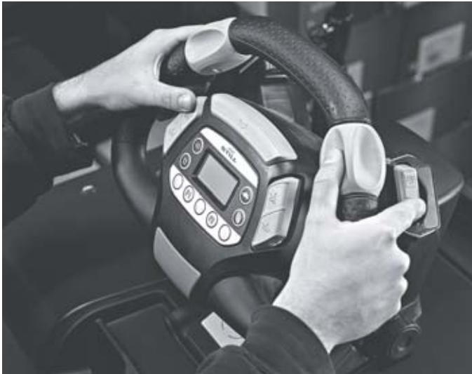
Unique STILL EASY Drive steering wheel for best driving experience and control of all functions without changing grip
