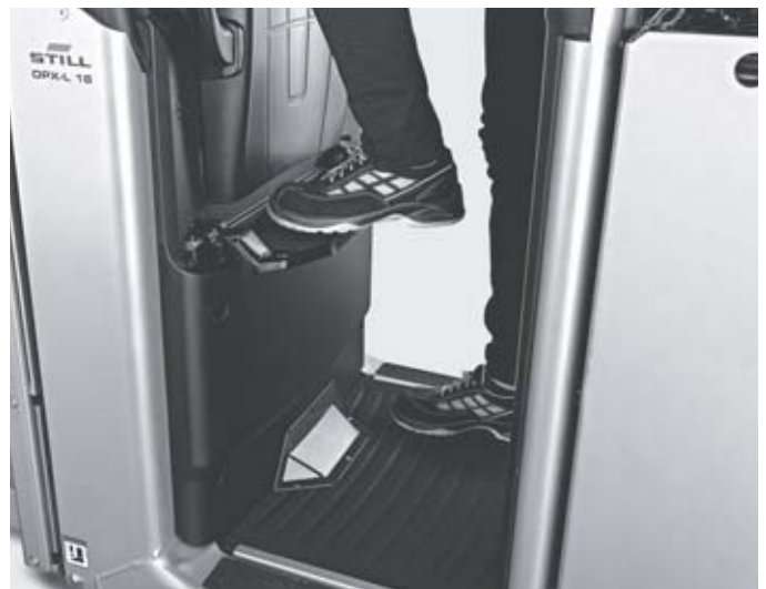
Optional foldable step for sporadic picking at first level
