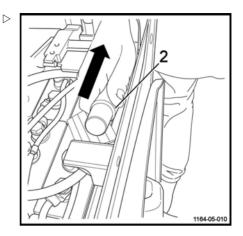
Lift the locking bar (3) until the battery is freed.
